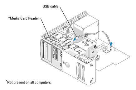
Disconnect the USB cable on the back of the Media Card Reader to the front panel USB connector on the system board (see page 63) and route the cable through the clip on the shroud.
