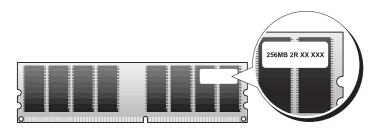
**NOTE:** Always install memory modules in the order indicated on the system board.
