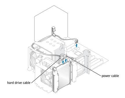
**2** Press in on the tabs on each side of the drive and slide the drive up and out.
