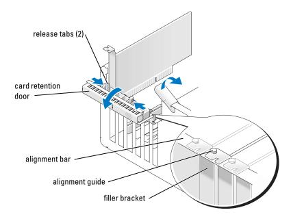
**3** Push the two release tabs on the card retention door from the inside to pivot the door open. Because the door is captive, it will remain in the open position.
